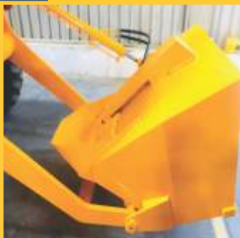
V- Shape articulated bucket with Hydraulic Shutter Gate to avoid spillage & better loading.
