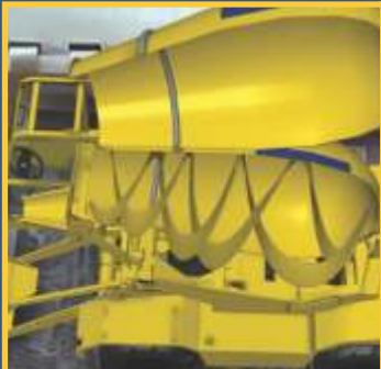
Double Helical Arrangement with low inclination of drum for better mixing.
