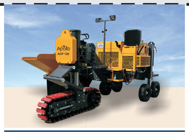
The ACP 120 is an ergonomically designed, easy-to-operate, slip form curb-laying machine. Its features enable the uniform placement of curbs in regard to leveling and shape. The machine, which can lay continuous curbs of 575 mm x 750 mm, is mounted on steel tracks to ensure maximum stability and grade ability. It can work at a pace of 120 metres per hour. The ACP 120 has a side-mounted mould that is essential while working in varied applications.
